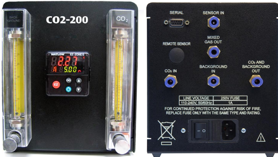
Fig. 1- The CO2-200 has both background and \text{CO}_2 flow meters on the front panel, as well as the PID controller. The back panel has the power switch and all the connection ports. The Remote Sensor port is not used on the CO2-200 .
