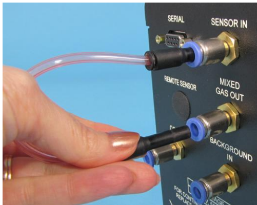
Fig. 4- Slide the tubing all the way into the port. In the image 0.156" tubing is used with quick fit reducers.
