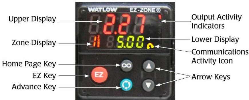
Fig. 2- The home page of the PID controller shows the actual percentage of CO 2 in the chamber and the setpoint.
