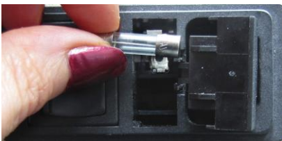
Fig. 10- Open the fuse housing and rotate it right to remove the fuse.
