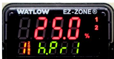
Fig. 4- The Watlow controller displays the percentage output.
