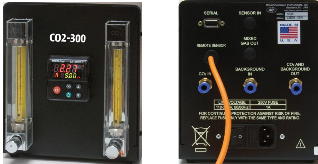
Fig. 1- The CO2-300 has both background and \text{CO}_2 flow meters on the front panel, as well as the PID controller. The back panel has the power switch and all the connection ports. The Sensor In and Mixed Gas Out ports are not used on the CO2-300 .
