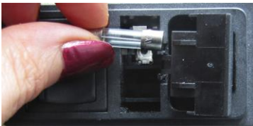
Fig. 9- Open the fuse housing and rotate it right to remove the fuse.
