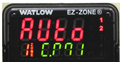
Fig. 6- The Watlow controller displays the control mode parameter.
